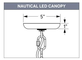
CHAIN LENGTHS: CN36 36", CN48 48", CN60 60", CN72 72" For custom lengths, please contact the factory.
