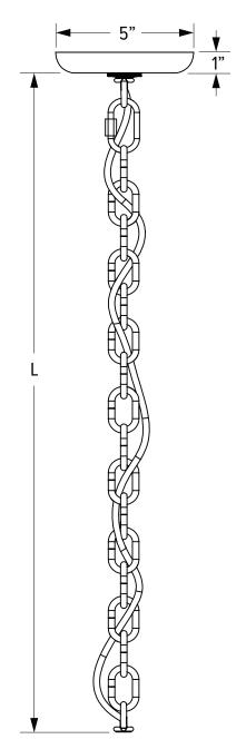
CHAIN LENGTHS: CN36 36", CN48 48", CN60 60", CN72 72" For custom lengths, please contact the factory.
