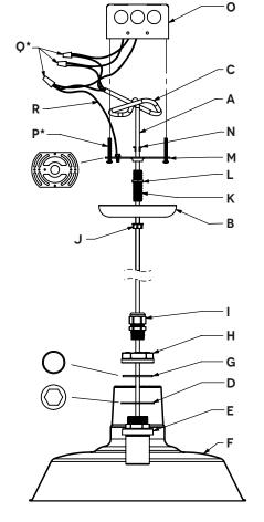
\*IMPORTANT: Mounting screws and wire nuts not included in hardware kit. Standard screw sizes include: 6-32, 8-32, 10-24 and 10-32.
