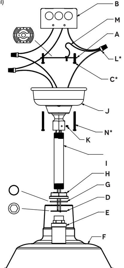
**\*IMPORTANT:** Mounting screws and wire nuts not included in hardware kit. Standard screw sizes include: 6-32, 8-32, 10-24 and 10-32.
